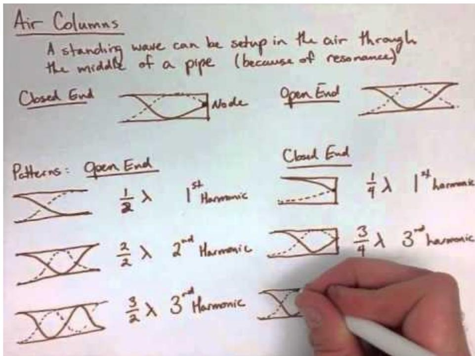
If you have ever played a wind instrument or listened to the sound of a guitar, you have probably encountered the concept of an air column. It is a hollow metal tube that is coiled a few times, nearly a meter long, with a small opening in the center that allows sound waves to pass through it. The open end allows sound to enter and exit the instrument. The air column in a musical instrument is a perfect example of an air column.
